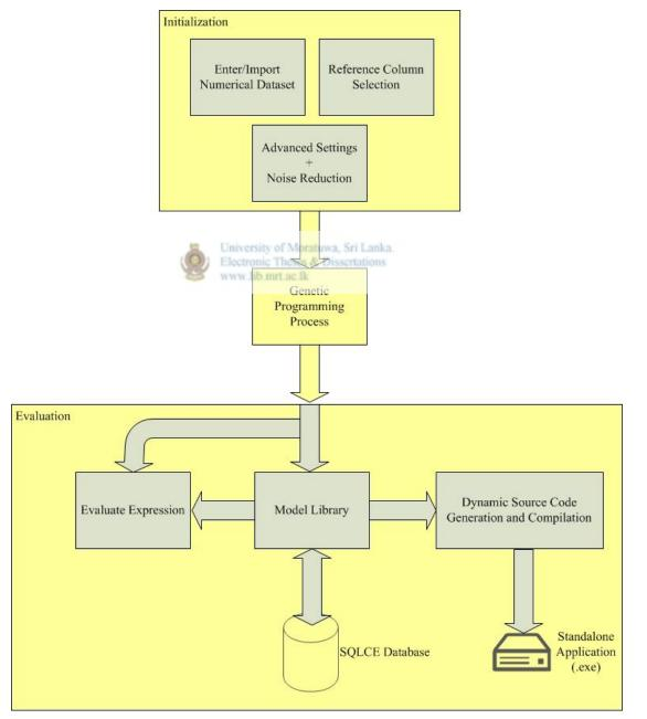
Figure A.1 – A detailed design diagram of GPVLab
