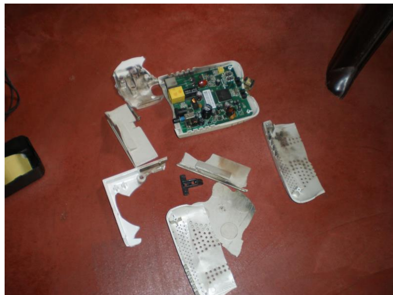
Figure 3.16: ADSL router damaged in home near the Thihariya site
