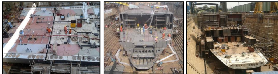
Figure 10: Unit Assembly process
