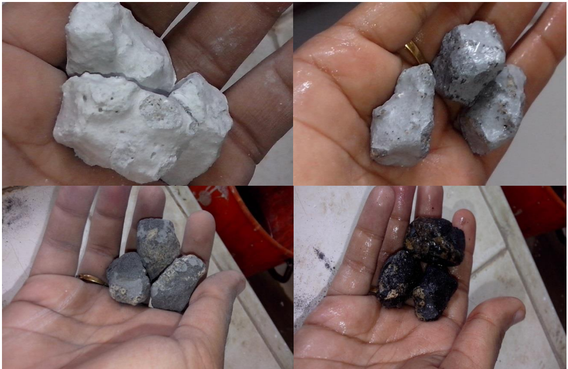
Figure 4. 29: Part of the coating obtained on the surface of RCA when using RHA-lime can be easily washed off after air drying it for 24 hours
