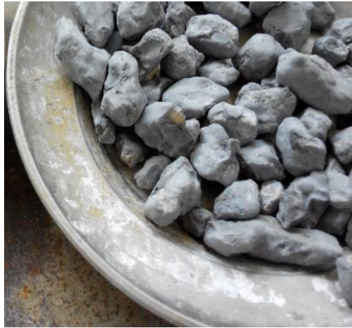
Figure 4. 34: A Treated RCA Sample [Slurry Ratio = 0.625, RHA (%): Cement (%) = 20:80]
