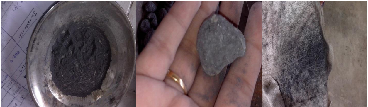
Figure 4. 30: Part of the coating obtained on the surface of RCA when using RHA-lime gets removed very easily
