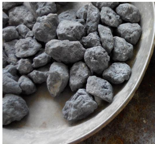
Figure 4. 33: A Treated RCA Sample [Slurry Ratio = 0.625, RHA (%) : Cement (%) = 40:60]
