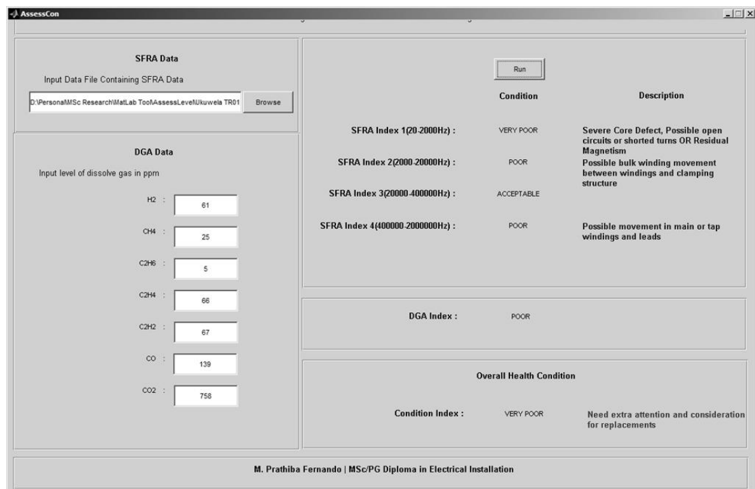
Figure 4.4: AssessCon condition prediction for failed Ukuwela TR01
