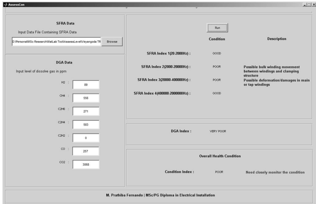
Figure 4.8: AssessCon condition prediction for Veyangoda TR02
