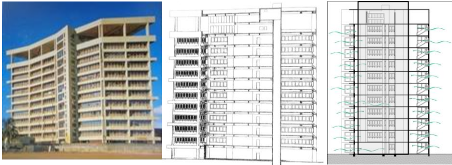
Figure 3: Sectional elevation through the building and Cross section through the north south plain to show the natural cross ventilation Source: (Robson D. , 2002) and Author
