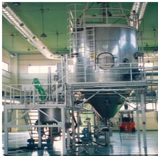
Figure 2-2: spray dryer used for powder preparation
