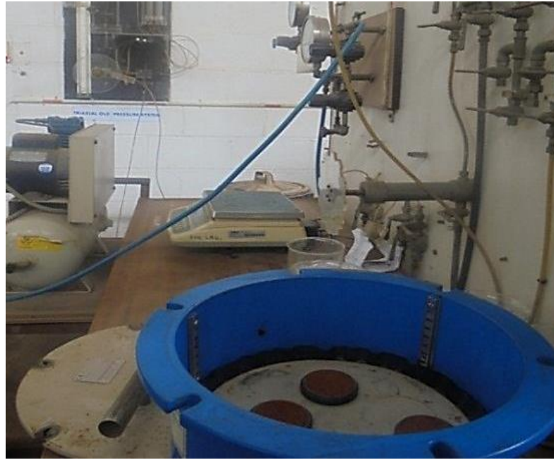
Figure 2.31: Typical arrangement of 5-bar pressure plate apparatus used for the research (Vasanthan 2016)
