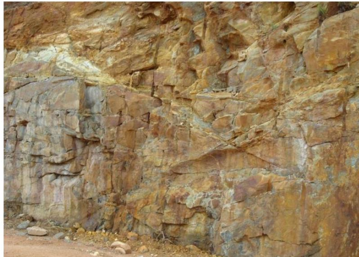
Figure2.8: Closely spaced rock Joints-remain as “Relict Joints” after weathering
