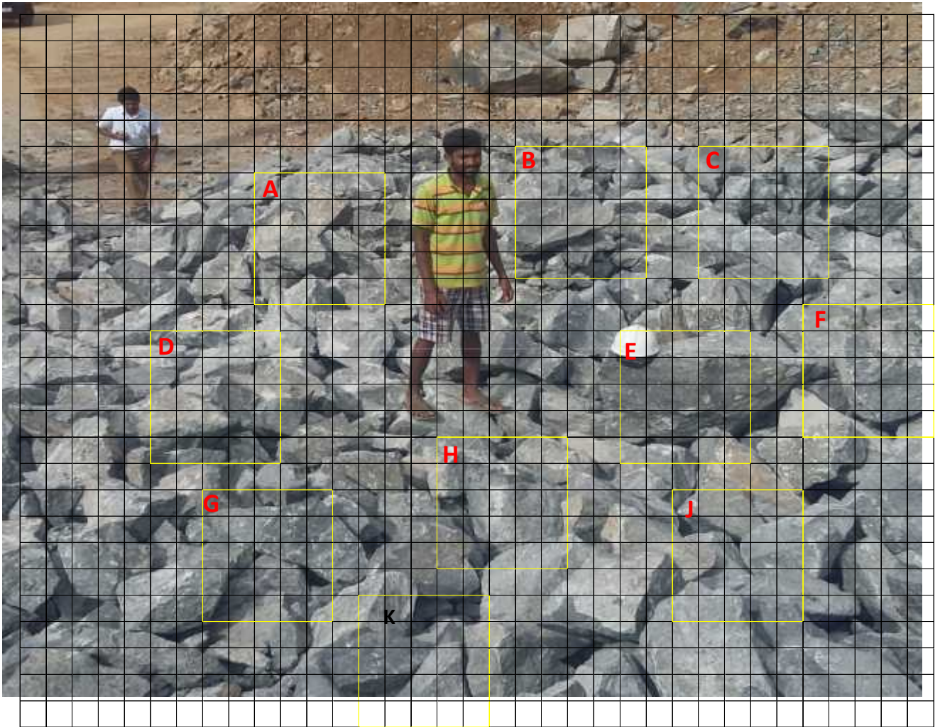
Figure 4.8 - analysis of samples using grid image in zone - G Scale 1 square : 100 cm 2
