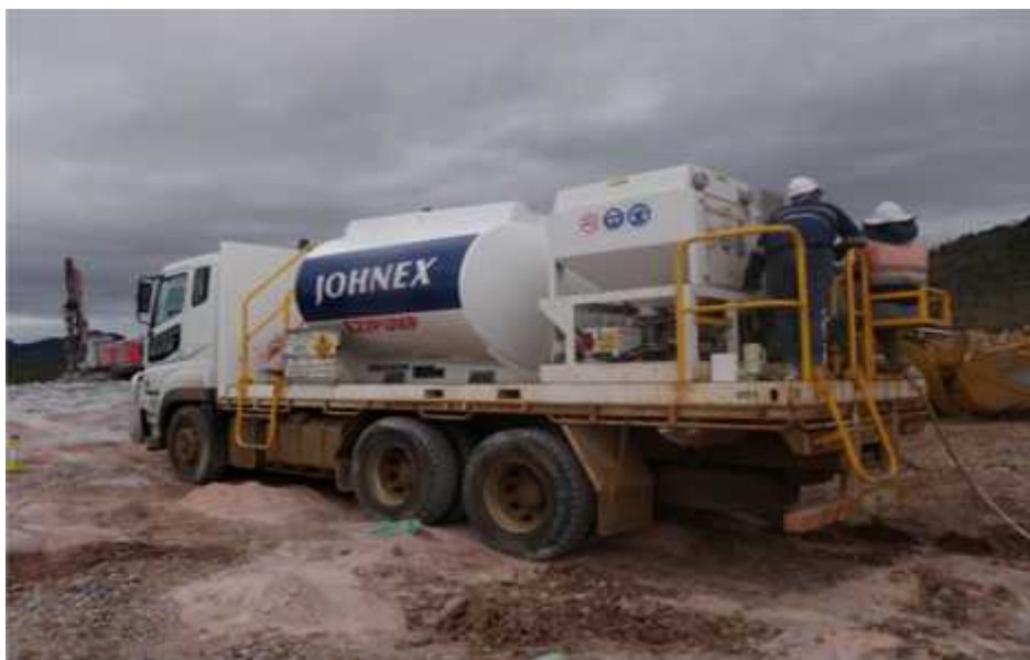
Figure 2.13: Image of bulk Emulsion Explosives loaded in a truck [8]
