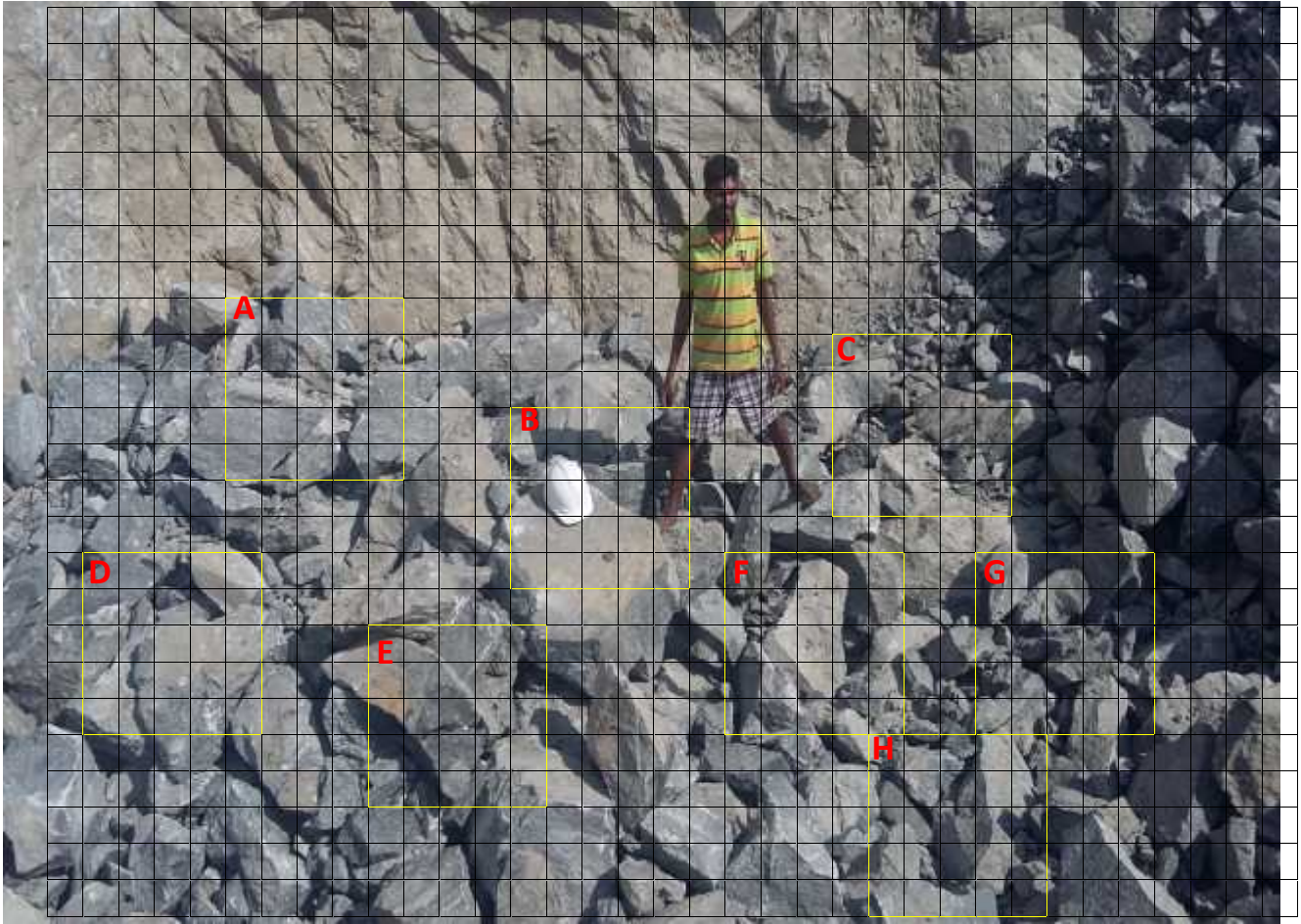
Figure 4.11 –Analysis of samples using grid image in zone - K Scale 1 square : 144 cm 2
