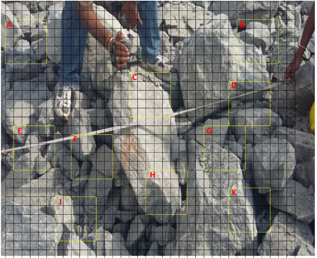
Figure 4.5. -Analysis of samples using grid image in zone - D Scale 1 square : 25 cm 2
