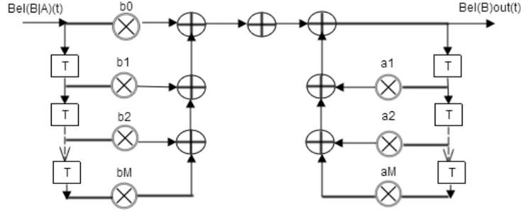
Fig. 5.1: Single Input Single Output Evidence Filter
