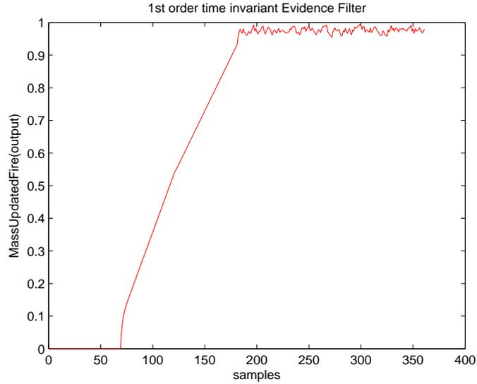
Fig. 3.4: First order Evidence Filter output
