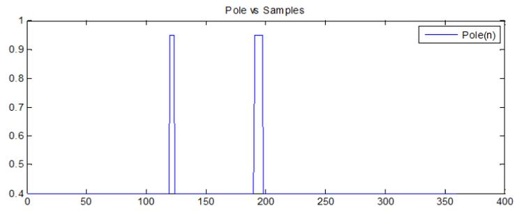
Fig. 3.7: Pole changes from .45 to 0.9
