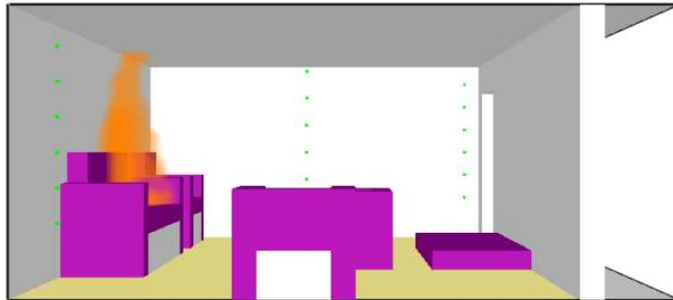
Fig. 4.1: Simulated room fire in FDS
