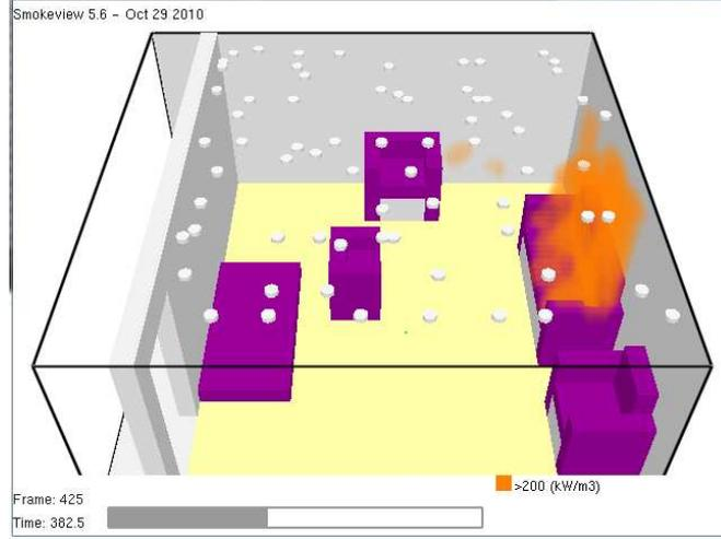
Fig. A.1: Simulation setup: Living room, Sensor nodes are deployed at the ceiling
