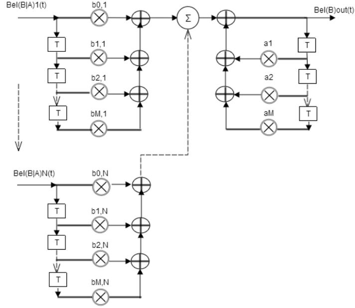
Fig. 5.2: Multiple Input Single Output Evidence Filter
