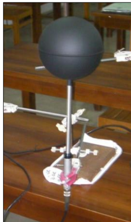
Figure 9.7: Black globe temperature sensor (Swema-05)
