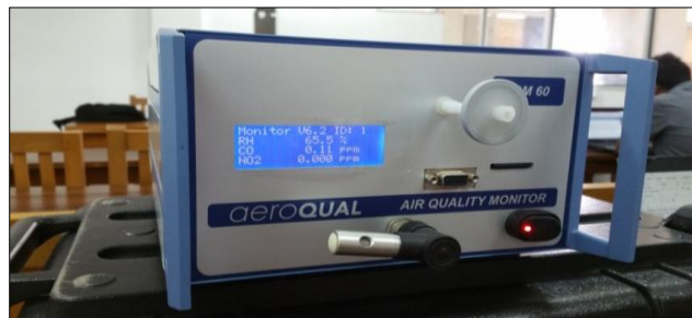
Figure 9.11: Indoor air quality monitor (IQM 60)
