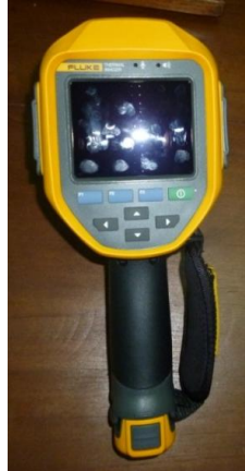
Figure 9.10: Thermal imaging camera (Fluke Ti400)
