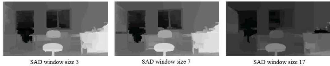
Figure 3.25 Disparity maps for different SAD window sizes
