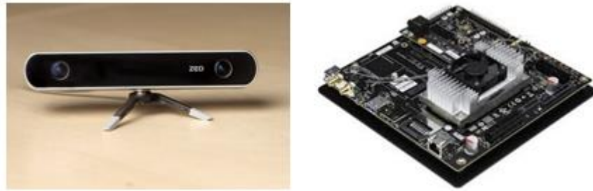
Figure 3.20 ZED stereo camera with Nvidia Jetson TX1 computing platform.
