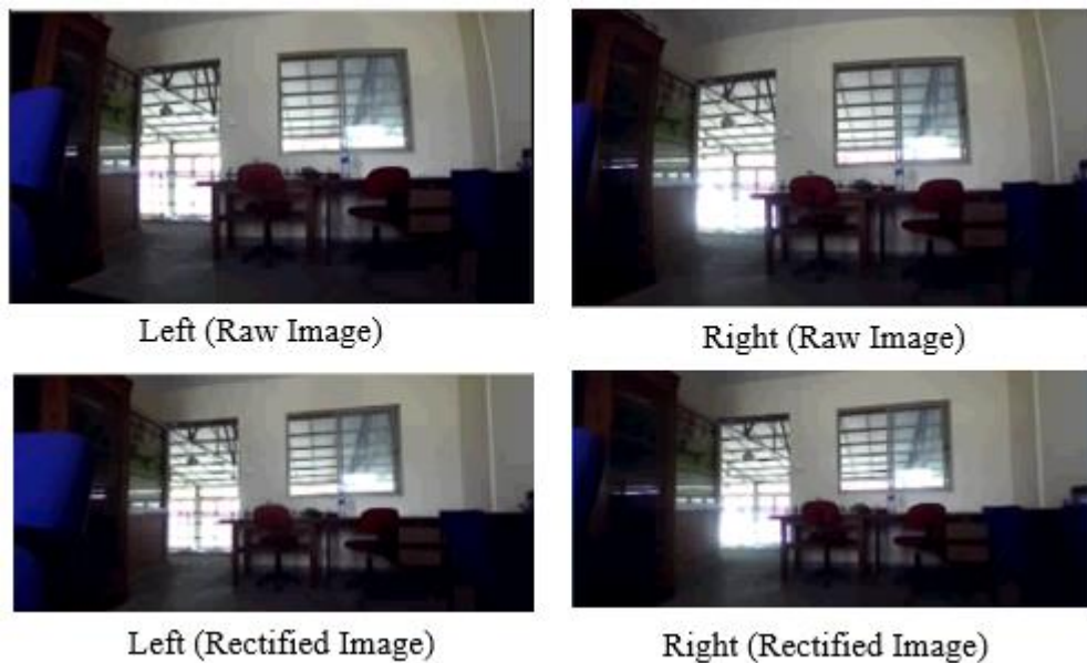
Figure 3.22 Raw images (Top) Rectified images (Bottom)
