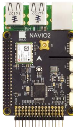
Figure 3.1 Navio2 flight shield connected with Raspberrypi 3 computer board.
