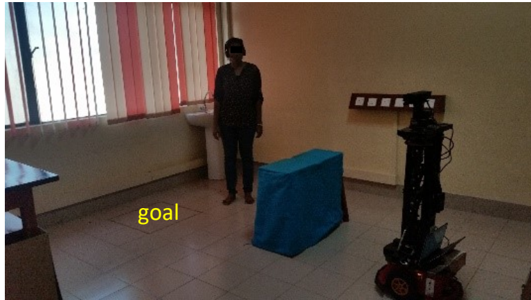
Figure 9.7: This shows the experimental scenario of the case 1 of the experiment for comparing the performance of the system with the MIS and the system without the MIS. The user was asked to navigate the robot to the goal position marked on the floor by implementing both the system in the robot. The goal area is annotated as “goal” in here.
