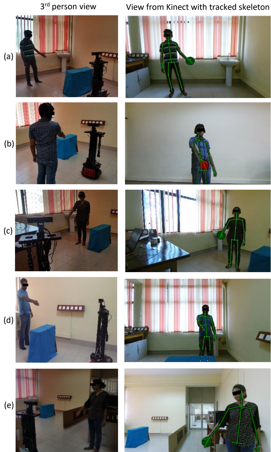
Figure 9.5: The view of the robot and the third person view of sample scenarios are shown with the corresponding case (a–e) given in Table 9.1. The tracked skeletons of the users are also superimposed with the RGB view of the robot for better clarity.
