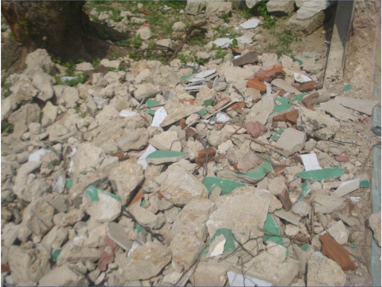
Fig. A7.4 Cement Plaster Debris
