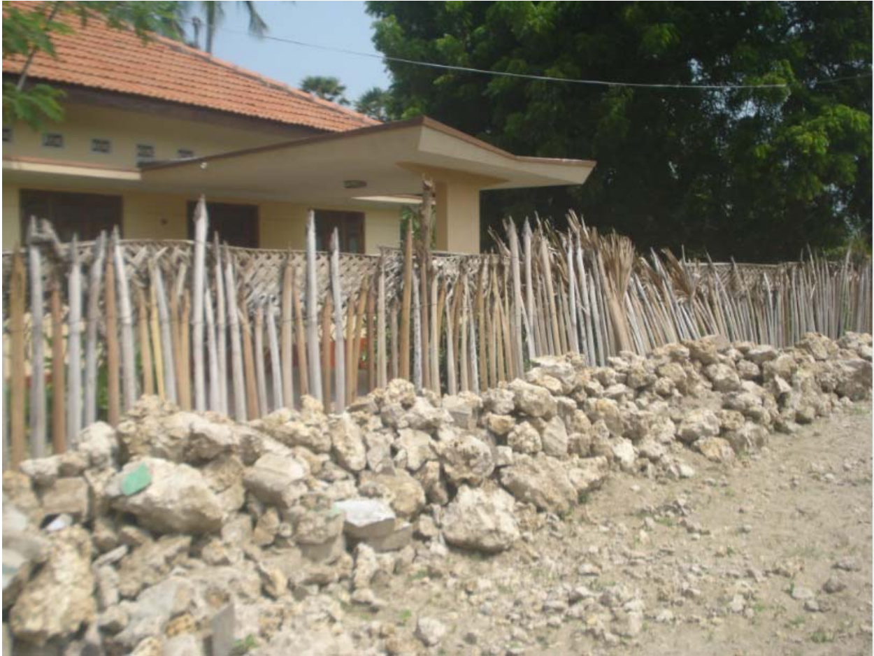
Fig. A7.3 Random Rubble Masonry Debris (Lime Stone)
