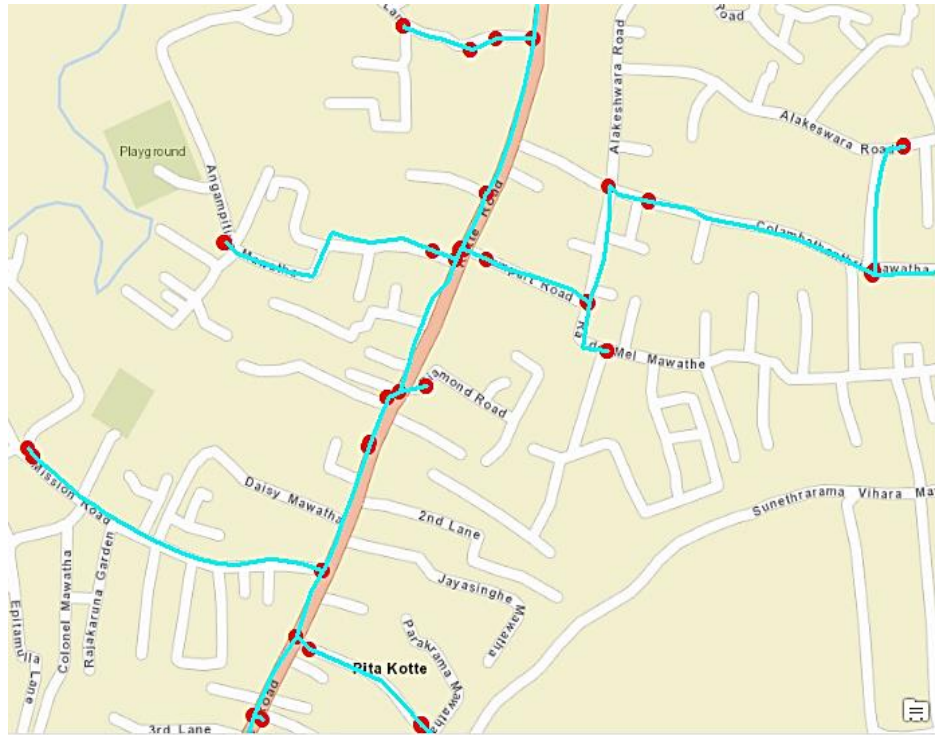
Figure 3.6: Located Nodes and the Splitted Lines
