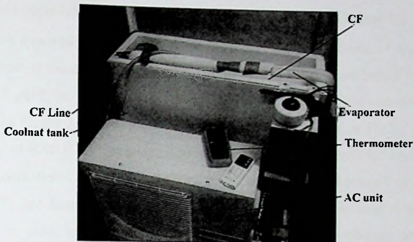
Figure 3.2: Fabricated cutting fluid cooling unit of the ACEMQL system
