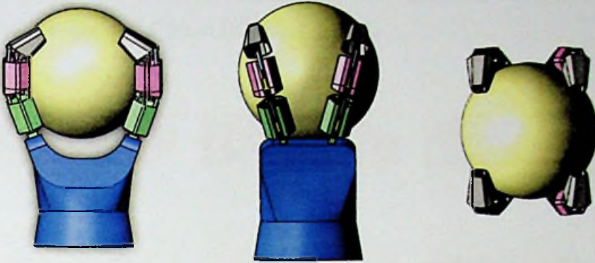
Figure 5.17: View orientations for 110mm diameter spherical grasp
