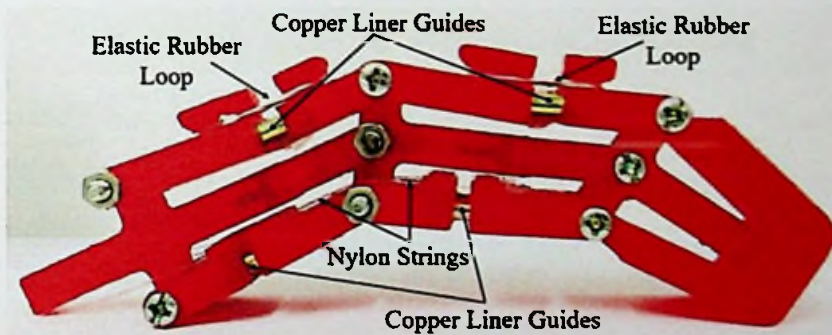
Figure 3.10: Fabricated finger mechanism
