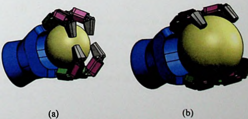
Figure 5.14: Spherical grasp of the prosthetic hand (a) 85mm sphere diameter (b) 110mm sphere diameter
