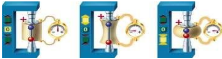
Figure 15: The direct piezoelectric effect [60].
