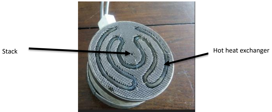
Figure 25: The stack and Hot heat exchanger
