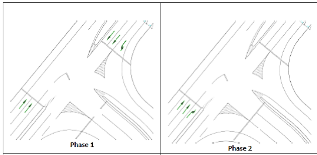
Figure 4-20: Phasing Arrangement for Intersection 4
