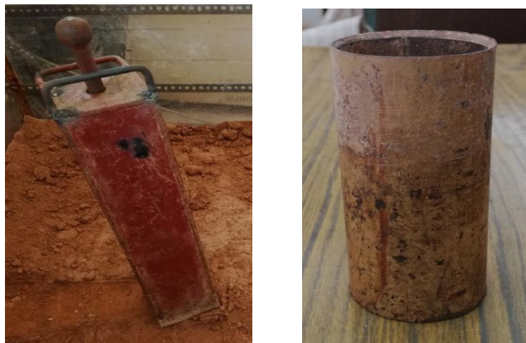
Figure 4.12 (a) Modified hammer (b) Modified core cutter
