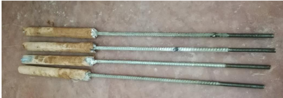
Figure 4.18 Completely pulled out soil nails.
