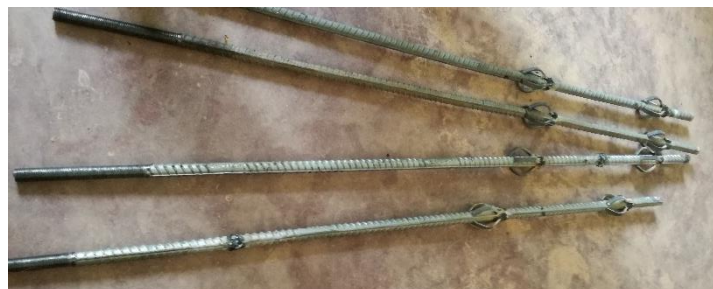
Figure 3.6 Soil nails with two centralizers
