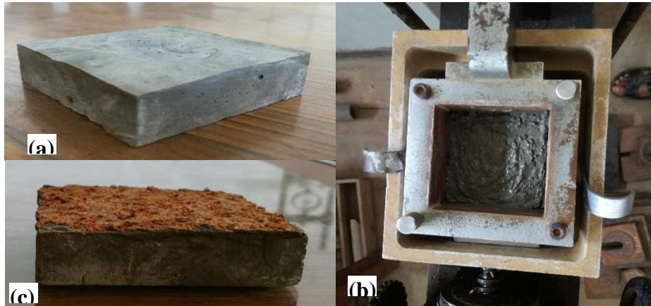
Figure 4.5 (a) The grout cube used in the interface test (b) The applied grout to the cube (c) The grout penetration zone
