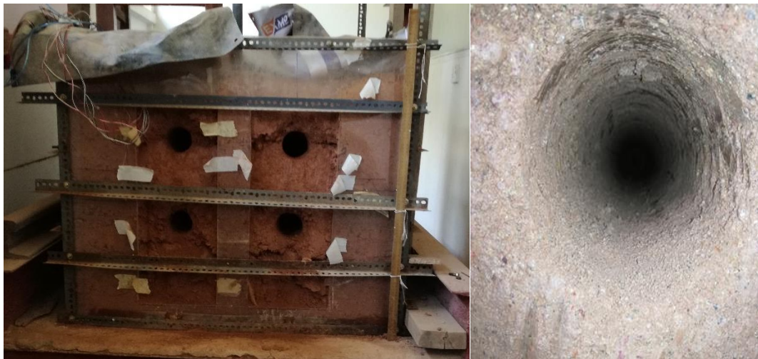
(b) Test box after drilling
