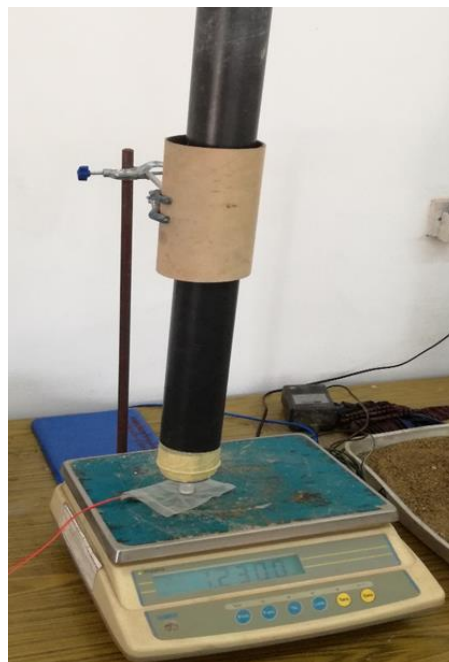
Figure 3.14 experimental arrangement for the Calibration of FSR
