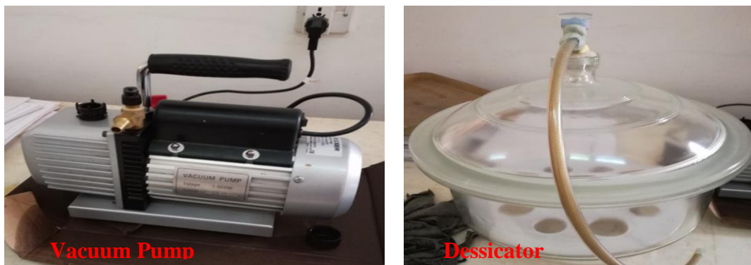
Figure 3.12 Equipment used for de-airing
