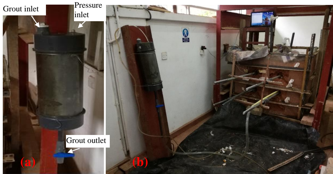
Figure 3.5 (a) The apparatus used for pressure grouting (b) The process of grouting.
