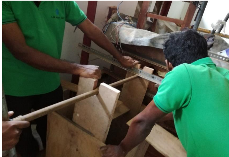
Figure 3.4 (a) Drilling of hole for soil nail installation
