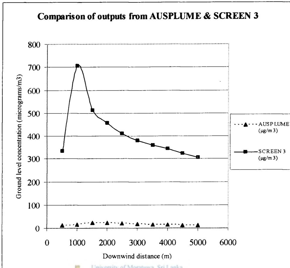
Figure 5.3: Predicted ground level; concentration of particulate matter using AUSPLUME and SCREEN 3
