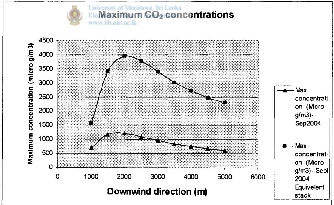
Figure 4.14: Distribution of maximum ground level concentrations of CO<sub>2</sub>
