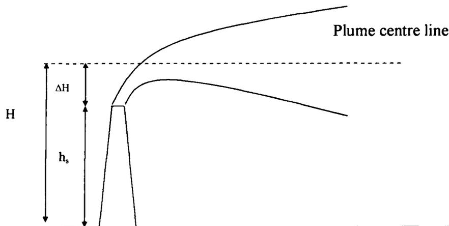
Figure 2.6: Height of a stack
