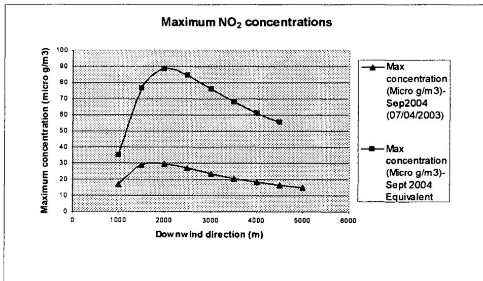
Figure 4.12: Distribution of maximum ground level concentrations of NO<sub>2</sub>
