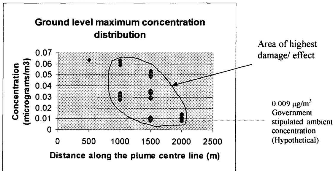
Figure 4.1: Ground Level Maximum Concentration for an Emission from a Stack Height 80m and Plume Exit Velocity 20m/s
