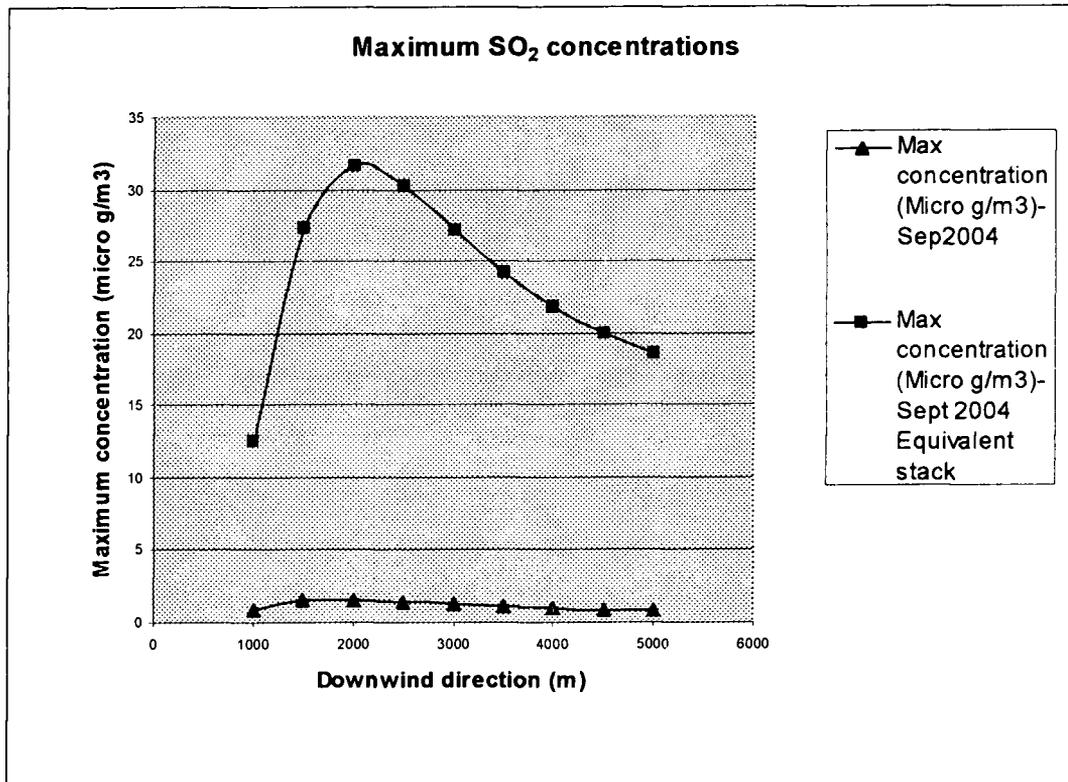
Figure 4.13: Distribution of maximum ground level concentrations of SO<sub>2</sub>
