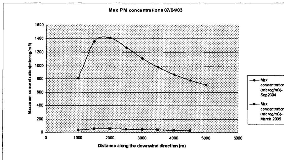
Figure 4.7: Distribution of maximum ground level concentrations of particulate matter
