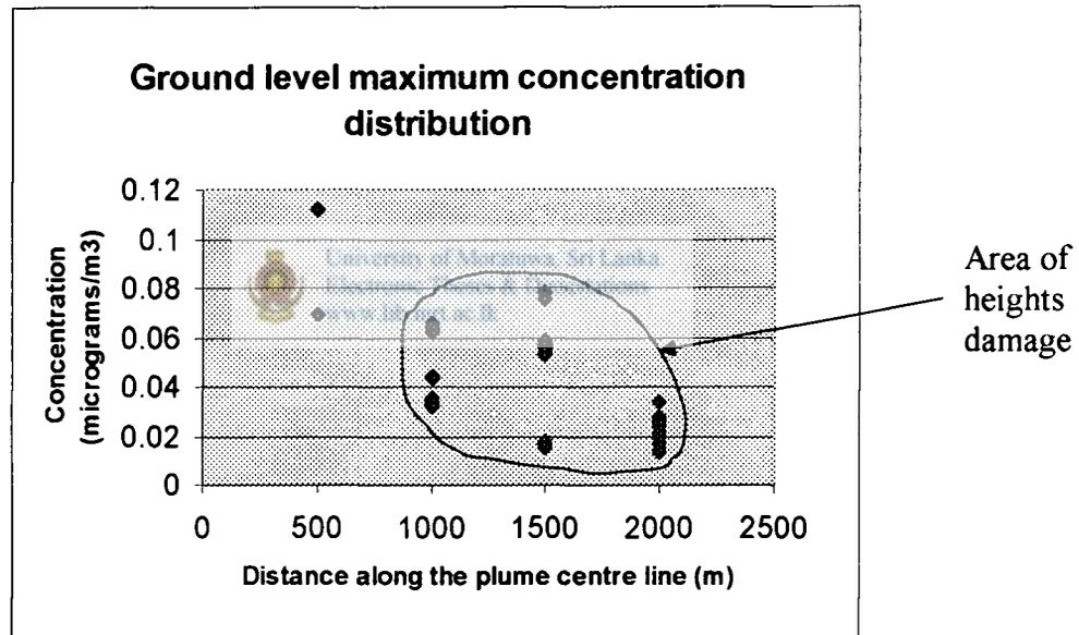
Figure 4.6: Ground Level Maximum Concentration for an Emission from a Stack Height 50m and Wind Velocity 25m/s
