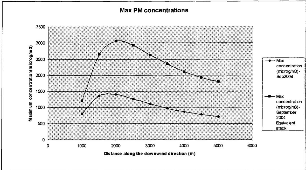
Figure 4.11: Distribution of maximum ground level concentrations of particulate matter
