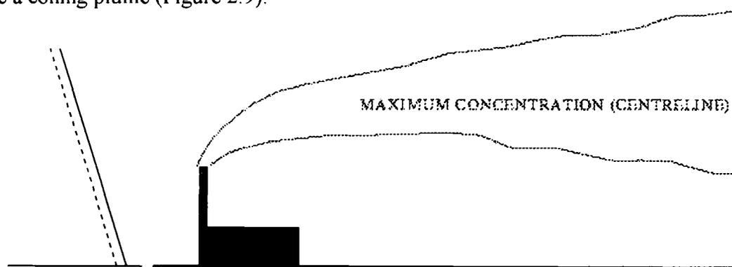
Figure 2.9: Coning Plume
