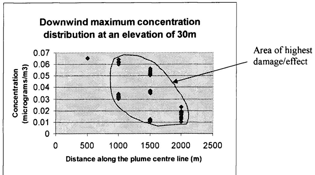
Figure 4.2: Maximum Concentration at a 30m Elevation for an Emission from a Stack Height 80m and Plume Exit Velocity 20m/s
