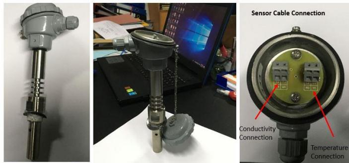
Figure 63: Sensor and Connection View of the Selected Sensor for the Project
