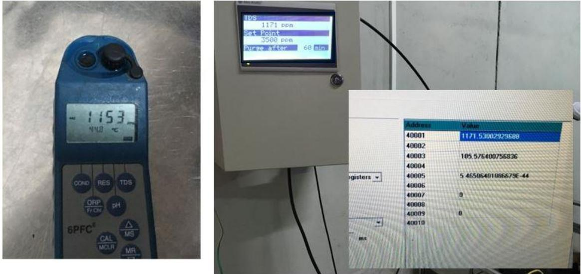
Figure 82: TDS Reading Comparison of Sensor Reading and Portable Meter Reading
