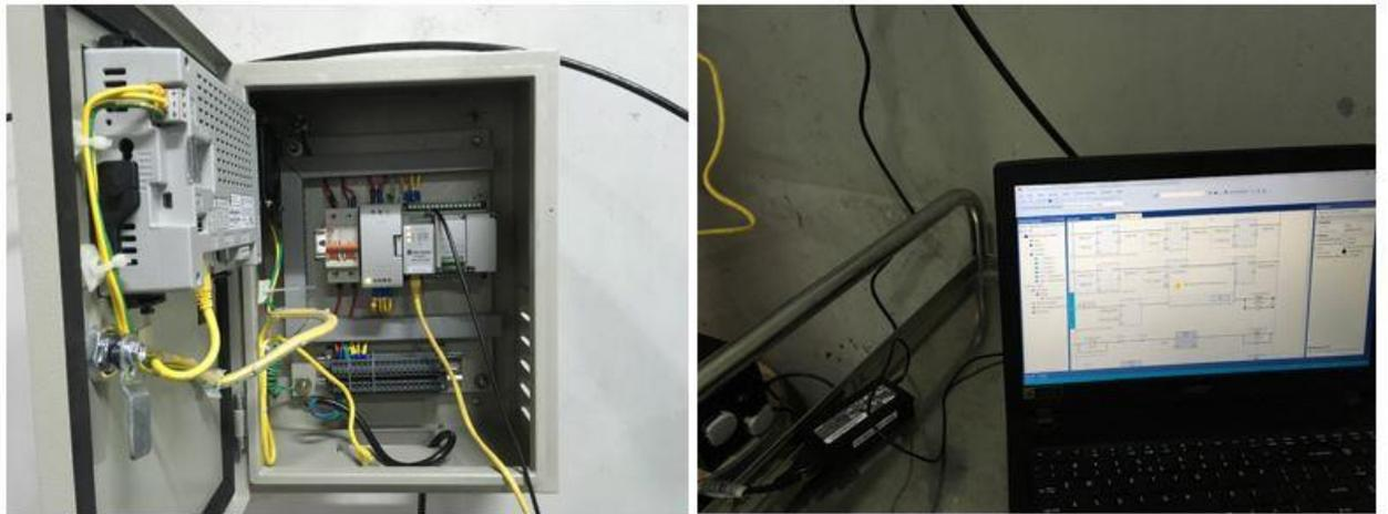
Figure 81: Testing and PLC Ladder Program Configuration
