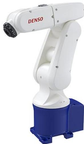
Figure 1.1: Denso robotics six degree of freedom robot manipulator model: VP 6242
