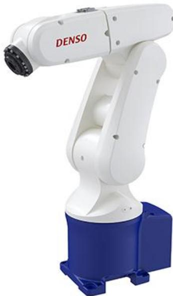
Figure 3.1: Denso VP 6242 mini sized vertical articulated robot
