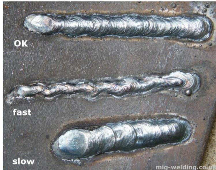
Figure 3.9: Arc welding defects due to speed changes [13]
