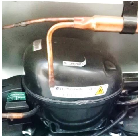
Figure 14: Compressor is the heart of the refrigerator
