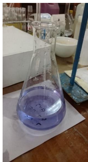
Figure A.25: Titration for Determining \text{NH}_4^+ - N (original in colour)
