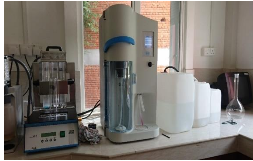
Figure A.27: “UDK 149 Automatic Distillation Unit – VELP” Kjeldahl Unit (original in colour)
