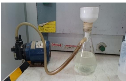
Figure A.28: Vacuum Filtering by the Buchner Funnel to Determine TSS (original in colour)
