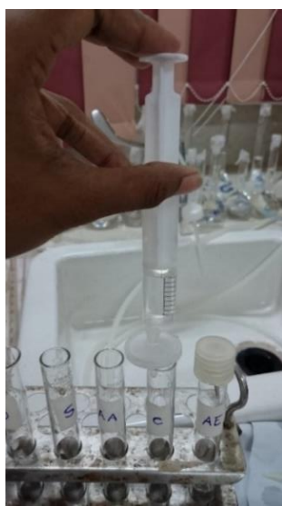
Figure A.24: Filtration by 0.45µm Syringe Filters (original in colour)
