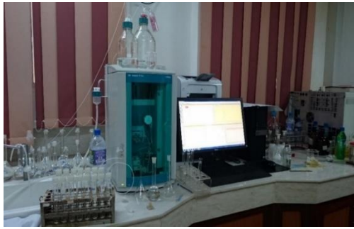
Figure A.26: “930 Compact IC Flex – MetroOhm” Ion Chromatography (IC) system (original in colour)
