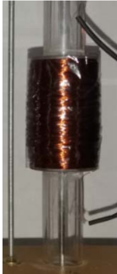
Figure 3.13: Stator winding of constructed Linear Generator
