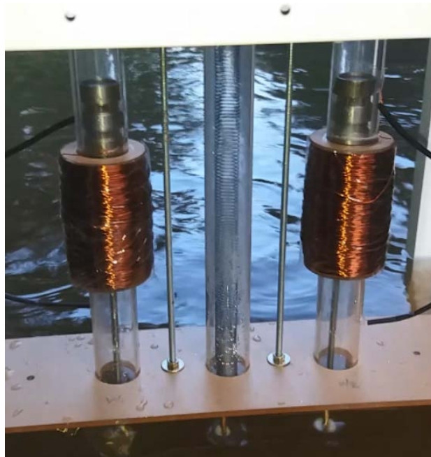
Figure 3.14: Implemented two identical generators
