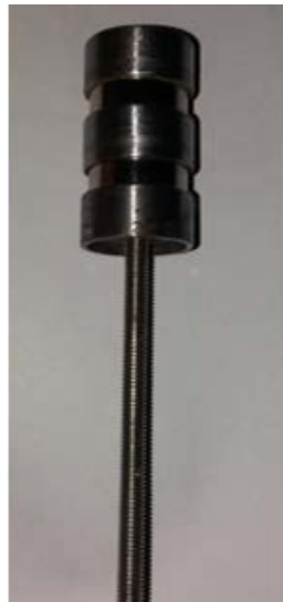
Figure 3.12: Translator of the constructed Linear Generator
