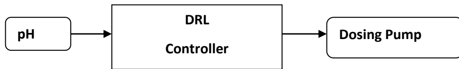
Figure 3.1 Relationship between the input and output of the DRL controller
