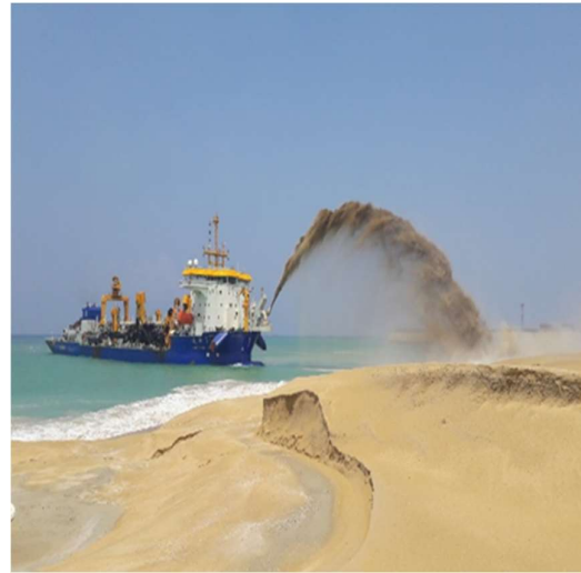
Figure 2-2: Sand Rain bowing from TSHD
