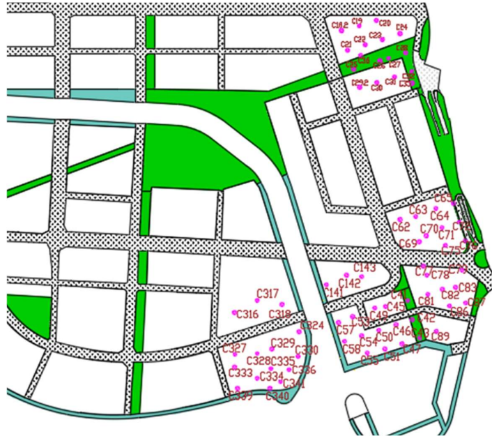
Figure 4-29: CPT locations in 2000kNm applied area
