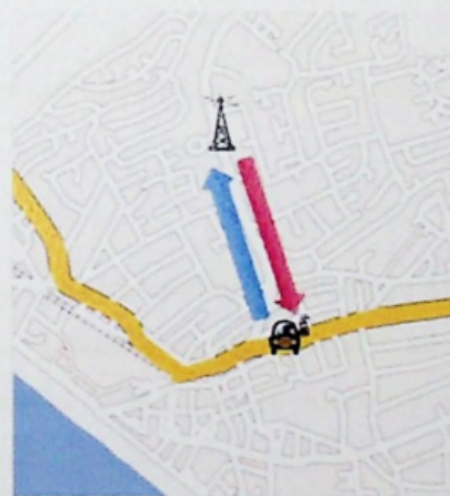
(b) Pull-based Dissemination. Vehicles request custom information from a nearby base station. The information is then routed back.
