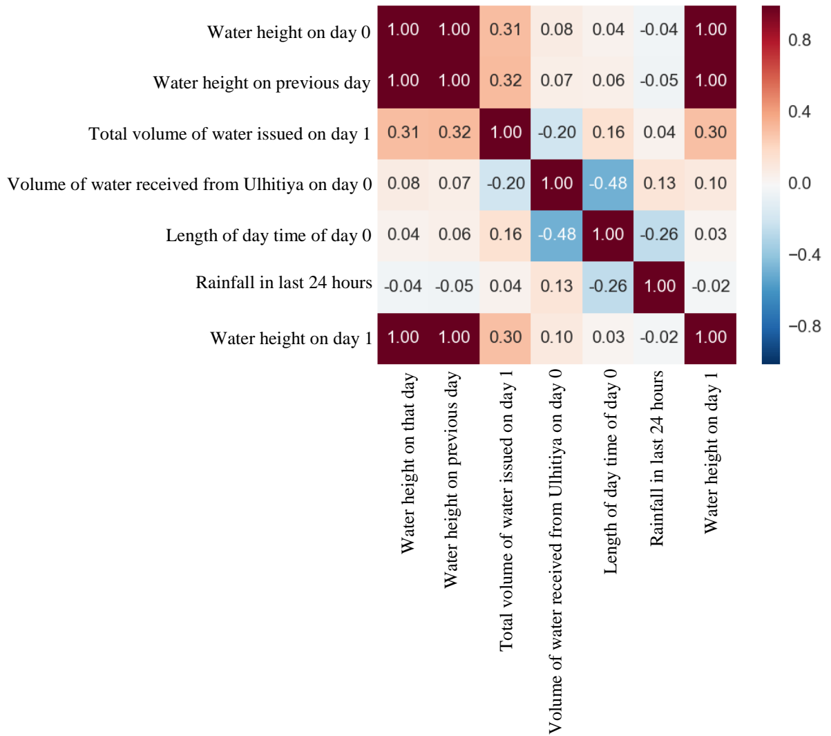
Fig 5.1 Correlation coefficients of the features to predict the water height on day 1
