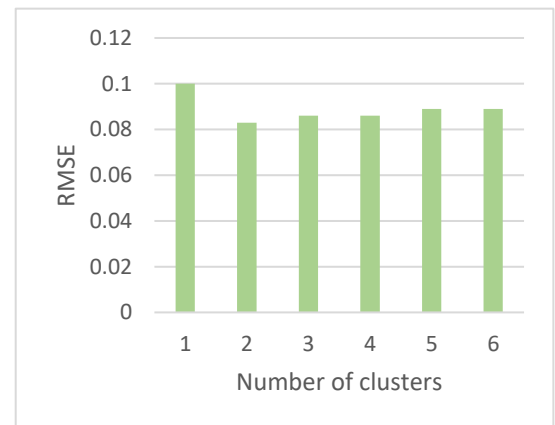
Fig 5.9 Variation of RMSE of predicted water height of linear regression model on day 2 with number of clusters on test data set
