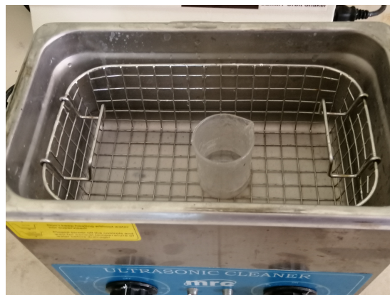
Figure 4.6: Dispersion of nano-particles inside the ultrasonic water bath.
