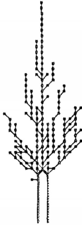
Figure 2.6: Example of a discharge structure with an internal electric field [82].
