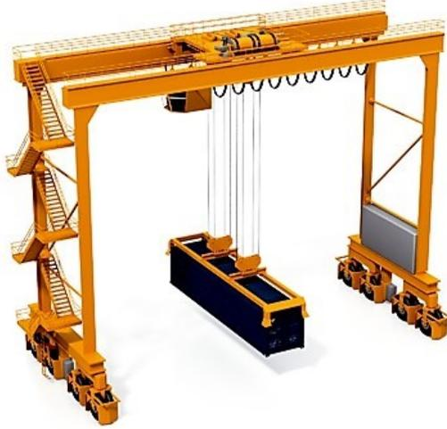
**Figure 2.2 :** Parallel rope arrangement
