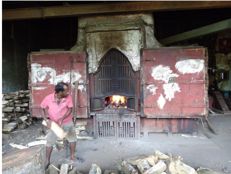
Figure 1.1 Packed bed wood burning furnace used in tea industry
