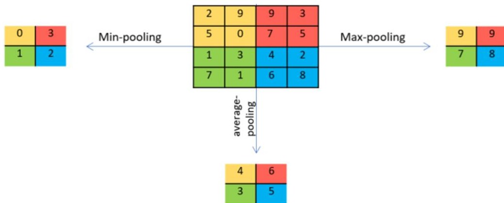
Figure 2.10: Visualisation of min, max, and average pooling
