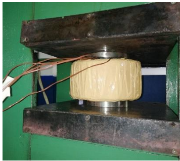
Figure 3-4 Curing the rubber block inside the press
