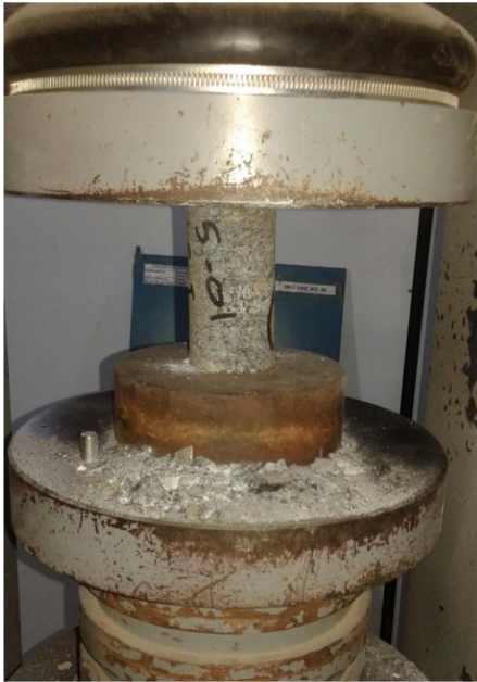
Figure 3.4: Conducting Unconfined Compression Test on the prepared rock core specimens
