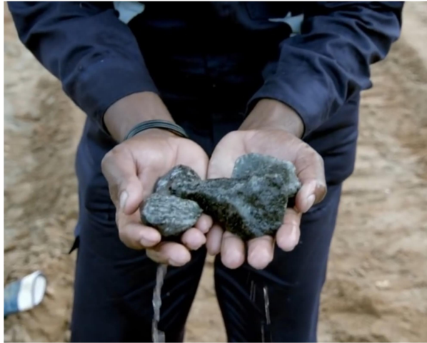
Figure 1.2: Nature of the rock samples recoverable during pile coring
