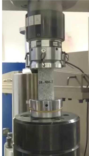
Figure 2.4: Typical machine used to conduct the Unconfined Compression test
