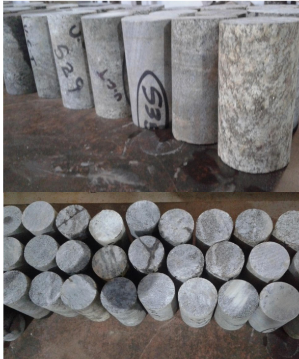
Figure 3.2: Preparation of rock samples for Unconfined Compression Test
