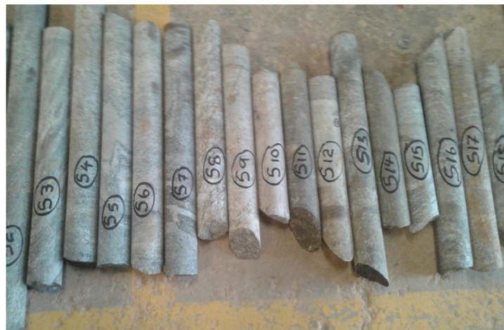
Figure 3.1: Some of the rock core samples collected from bore hole investigation sites. The collected rock cores were grouped into different types of rocks. Thereafter, the rock cores were prepared for laboratory testing.
