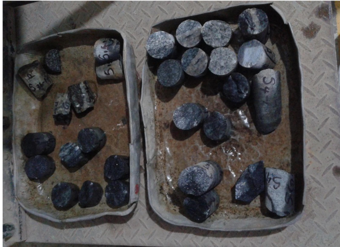
Figure 3.6: Rock core samples prepared for Specific Gravity Test
