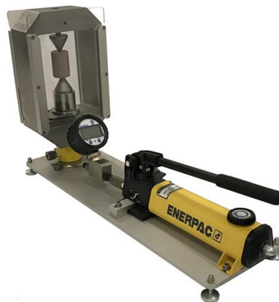
Figure 2.3: Typical machine used to conduct the Point Load Strength Index test (Source: http://www.floxlab.com/plt-100-point-load-tester-41.aspx )
