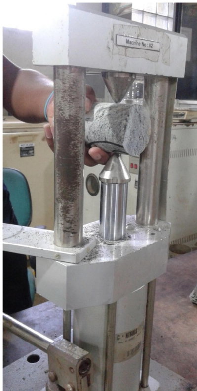
Figure 3.5: Conducting Point Load Index Test on the prepared rock core specimens
