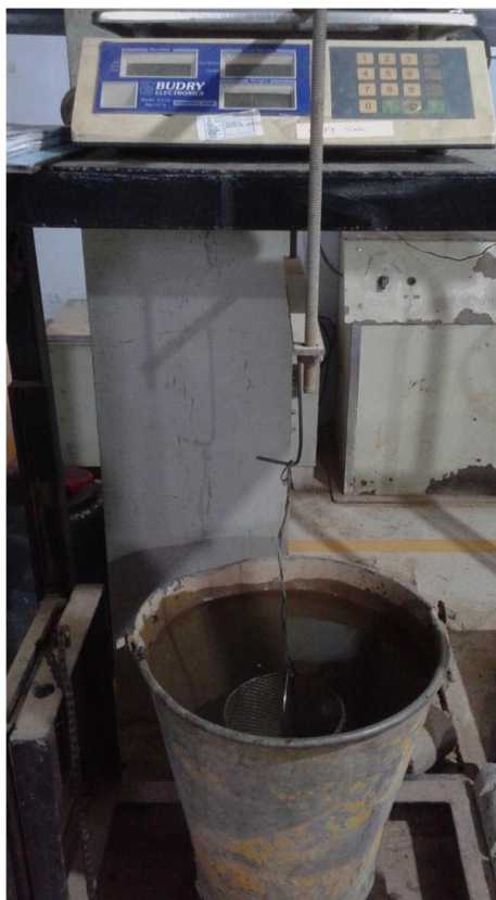
Figure 3.7: Conducting Specific Gravity test on rock samples as per the wire basket method
