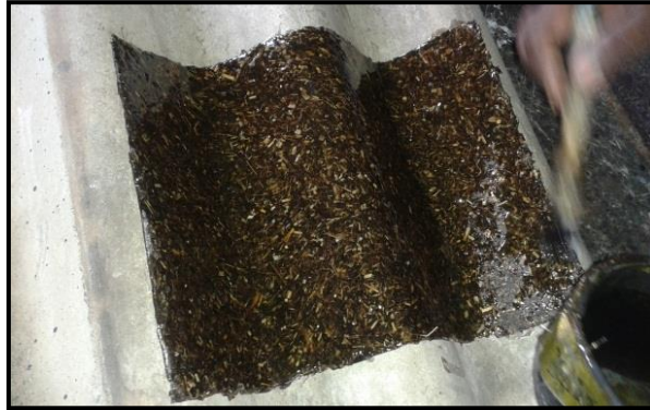
Figure 1.1: Trial product with rice husk-polyester composite
