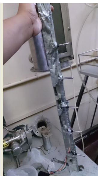
Figure 3.4: Arrangement of temperature sensors inside the spouted bed contactor
