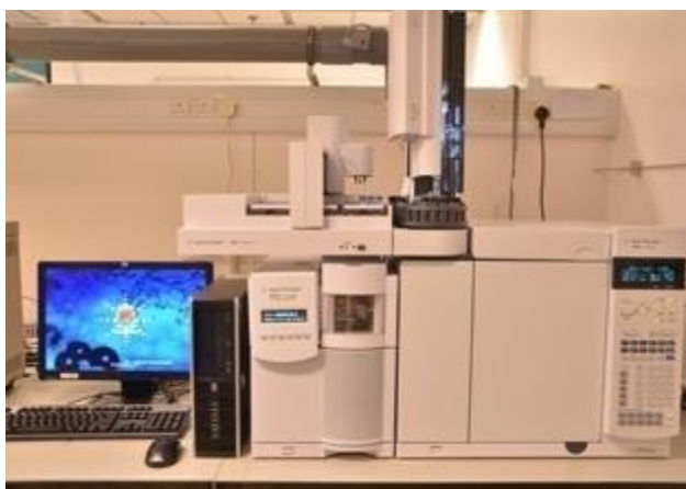
Figure 5: GC-MS)-7890A gas chromatograph (Agilent, American) equipped with a 5975C plus mass spectrometer (Agilent, American)
