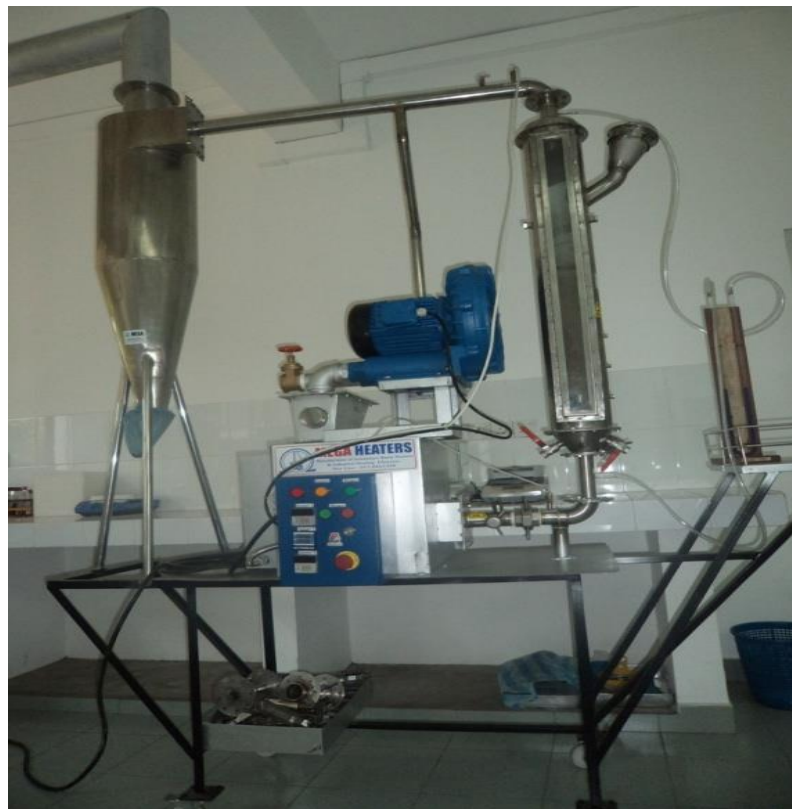
Figure 3.3: Image of spouted bed drying experiment set up
