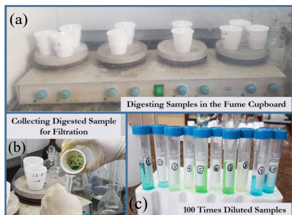
Figure 3: Digestion Process ((a) Digesting samples in the fume cupboard; (b) Collecting digested samples for filtration; (c) 100 times diluted samples).
