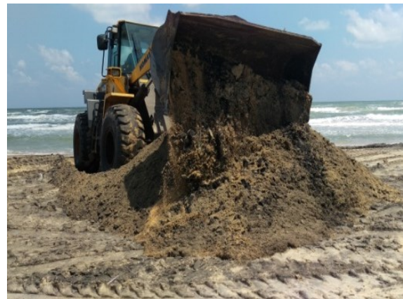
Figure 8: Mechanical scraping operation at Pulmoddai using wheel loader.
