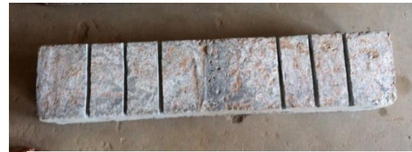
Fig. 1 Grooves prepared perpendicular to main steel reinforcement (at the bottom face)
