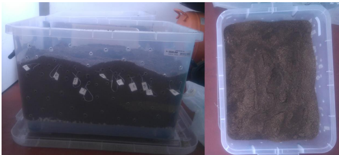
Figure 3.1: Test assemblies of soil burial test
