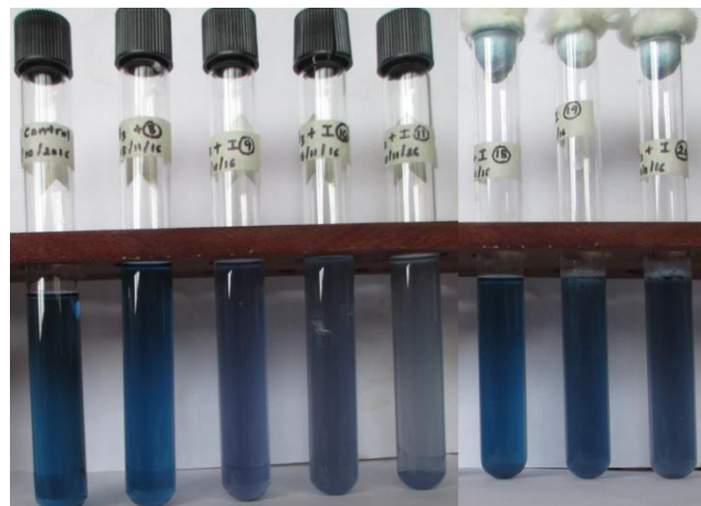
Figure 4.13: Blue EXF dye containing nutrient media inoculated with isolates 8, 9, 10, 11, 18, 19 and 20 after 10 days of incubation and control (first tube starting from left hand side)
