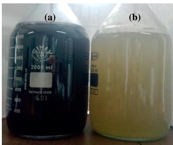
Figure 4.71: a) Influent (50 mg/l synthetic dye mixture containing medium) and b) treated water obtained during phase III operation of FBBR
