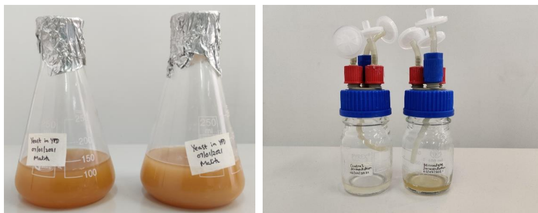
Figure 3-6: Seed cultures of S. cerevisiae prepared for fermentation of residual T. lutea biomass (left) and fermentation apparatus (right)
