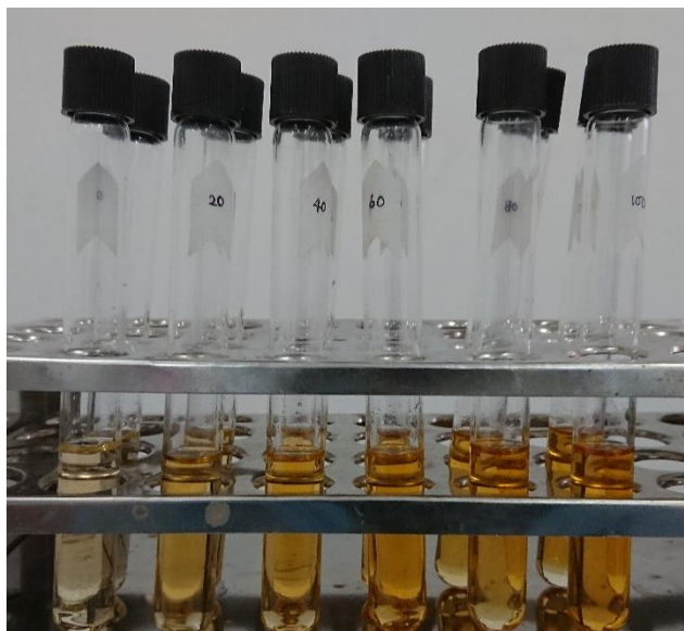
Figure 3-4: Color development in sugar hydrolysates upon the addition of phenol-sulfuric reagent for determination of carbohydrate concentration
