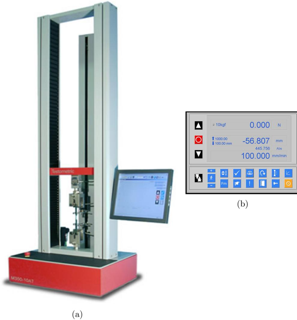
Figure 4.2: (a) Universal Testing Machine (b) WinTest Software Interface
