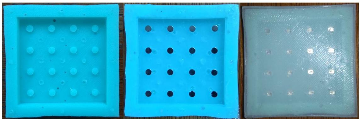
Figure 3.11: Steps in developing the elastomer from Left to Right – Outer Layer, Intermediate Layer & Magnets and Inner Layer
