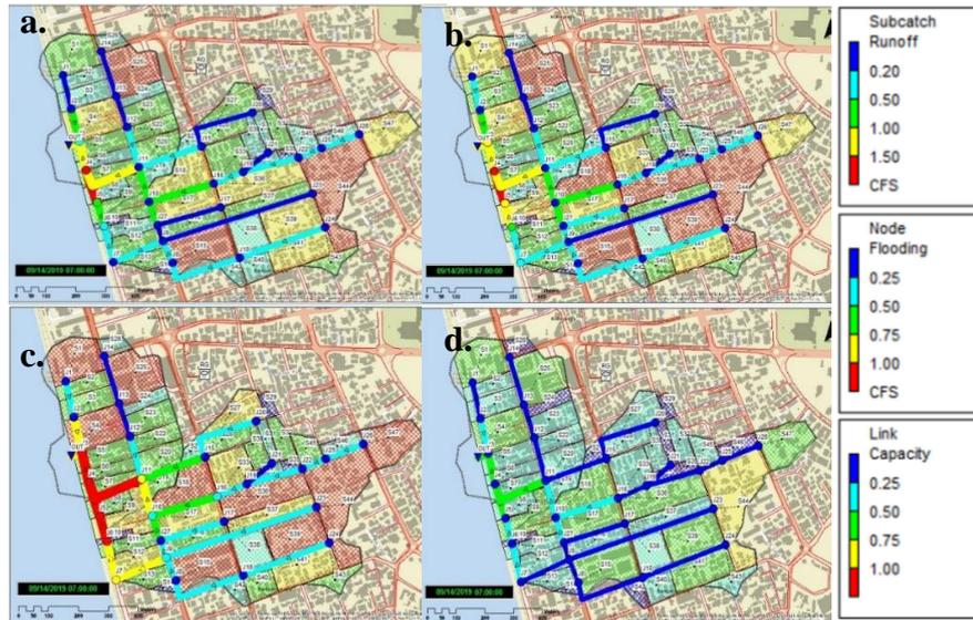
Figure 5: Runoff, node flooding and drainage capacity by changing imperviousness under scenario 1 to 4
