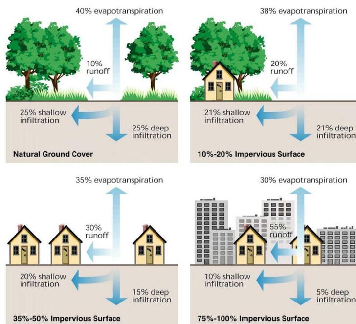
Figure 1: Effects of Imperviousness on Runoff and Infiltration
