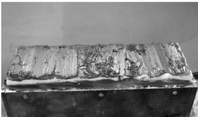
Fig. 8. Compacted and polished surface of graphite infill in some parts of the specimen after shearing
