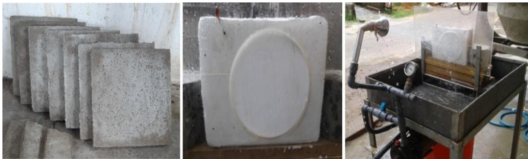
Figure 7.21: Sample preparation and spray erosion test for comparison of different wall finishes
