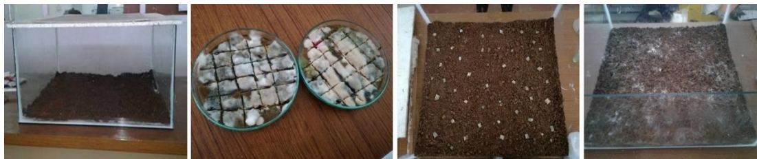
Figure 7.8: Fungus test chamber preparation
