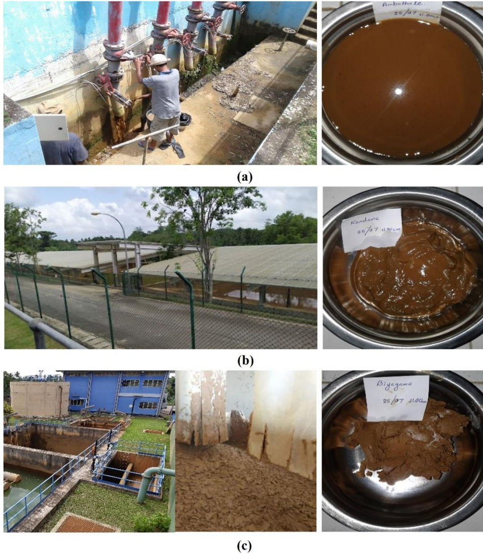
Figure 3.2: Collected sludge samples; (a) Raw sludge from Ambathale DWTP (b) Sludge from sludge drying beds in Kandana DWTP (c) Dewatered sludge from Biyagama DWTP
