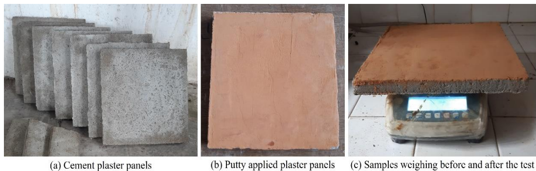
Figure 7.11: Sample preparation for spray erosion test of sludge putty mixtures with stabilizers
