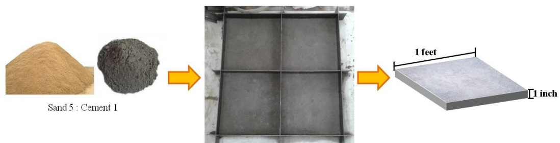
Figure 4.5: Sand cement plaster panel casting for observational shrinkage test
