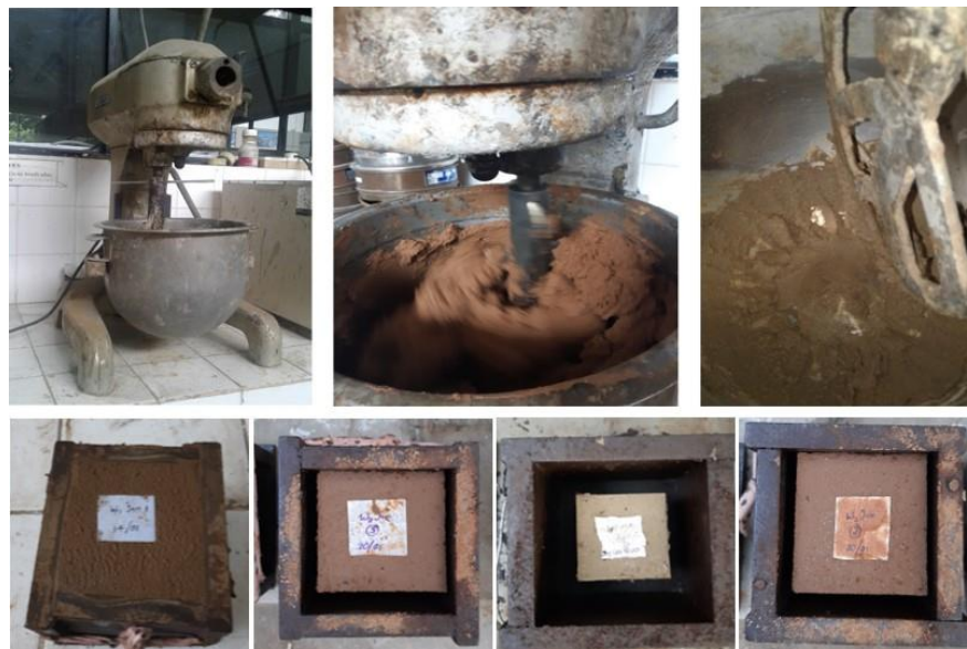
Figure 5.2: Mixing with mechanical mixer and cube casting for volumetric shrinkage test
