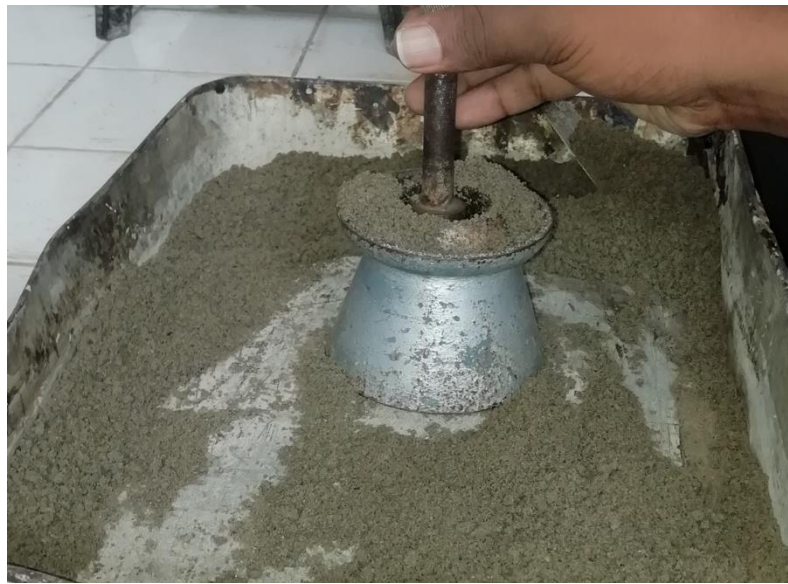
Figure 4.3 Identification of SSD condition of fine aggregates
