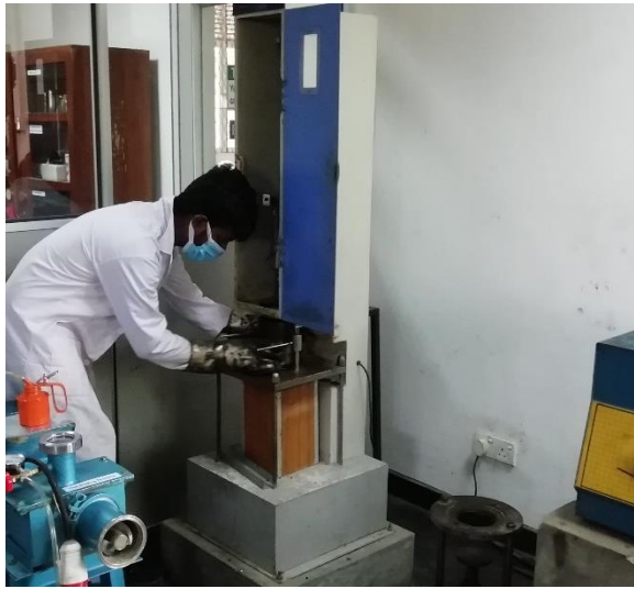
Figure 4.4 Preparation of Marshal samples
