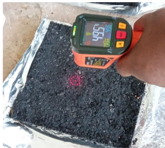
Figure 6.2 Measurement of temperature of sample using IR thermometer
