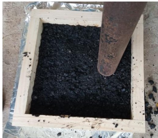
Figure 6.1 Preparation of sample on slab mould
