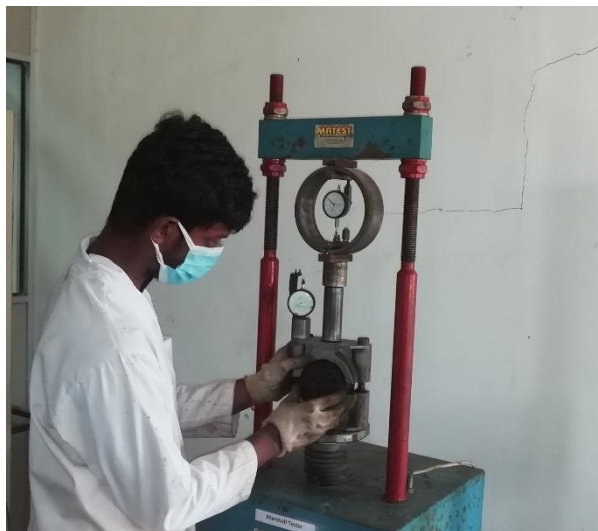
Figure 4.6 Testing of Marshal Samples
